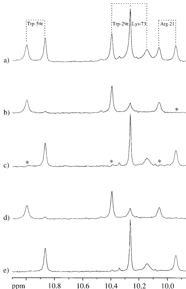
FIG. 2. ^{15}N -RAP 17-97 750-MHz Varian Unity Inova ^1H NMR spectra (part of amide region) (2.3 mM in 90%/10% H_2O/D_2O , pH 6.4, 20 mM NaCl, 1 mM phosphate buffer) recorded at 298 K with water presaturation and all representing 64 scans. The spectra represent (a) \pi/2 pulse excitation, (b) and (c) the S^3E sequence in Fig. 1b employing a delay of \tau = 5.26 ms with the first and third entries, and (d, e) all four steps of the phase cycles in Table 1. Asterisks indicate residual dispersive cross talk between the edited subspectra.
